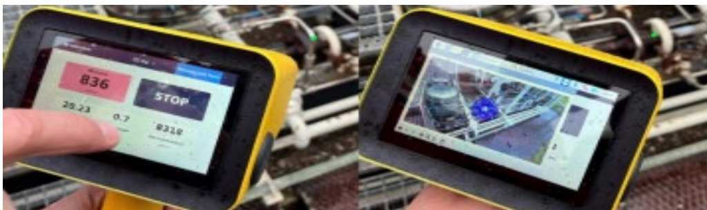
Figure 2. Detection of the emission (concentration above 500ppm-m) and visualization of the emission otherwise not visible to the naked eye by the Xplorobot Laser OGI device.
