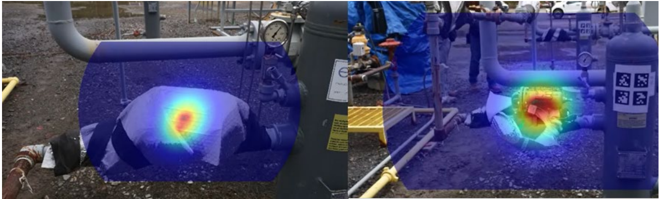
Figure 10. Emissions were detected under a bubble wrap, and the recording on the regulator after the wrap was removed.
