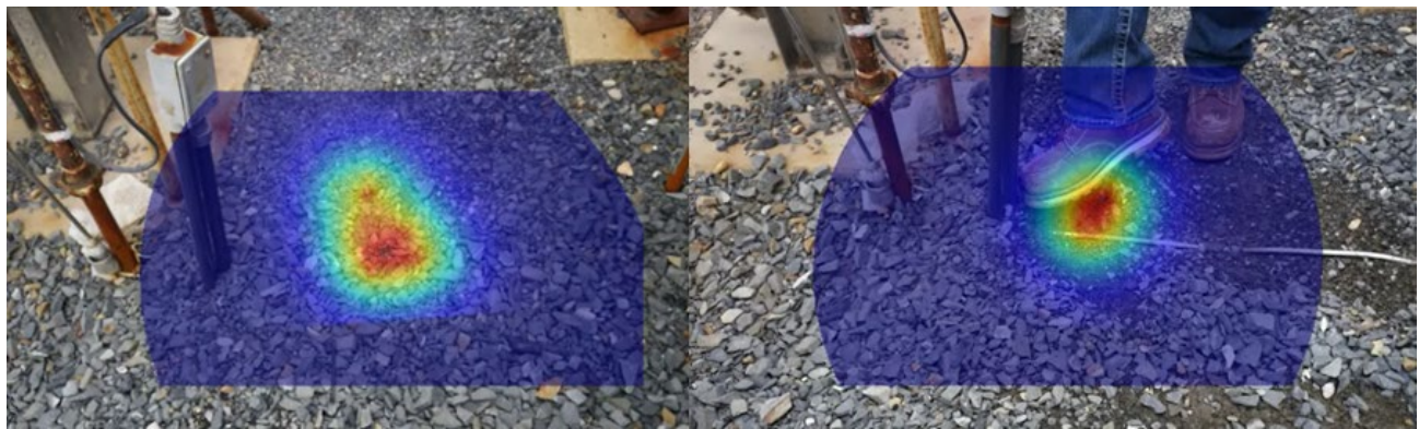
Figure 11. Emission detected under gravel and recorded on tubing after gravel was removed.
